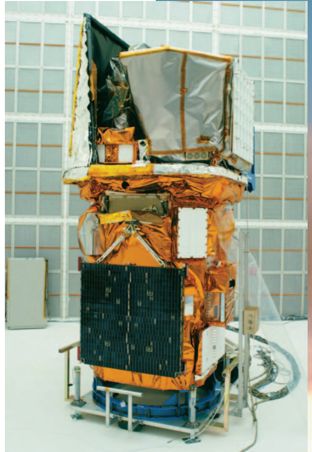
Fig 3a: The Swift satellite, equipped with gamma-ray, X-ray, and optical cameras for immediate localisation of GRBs.
